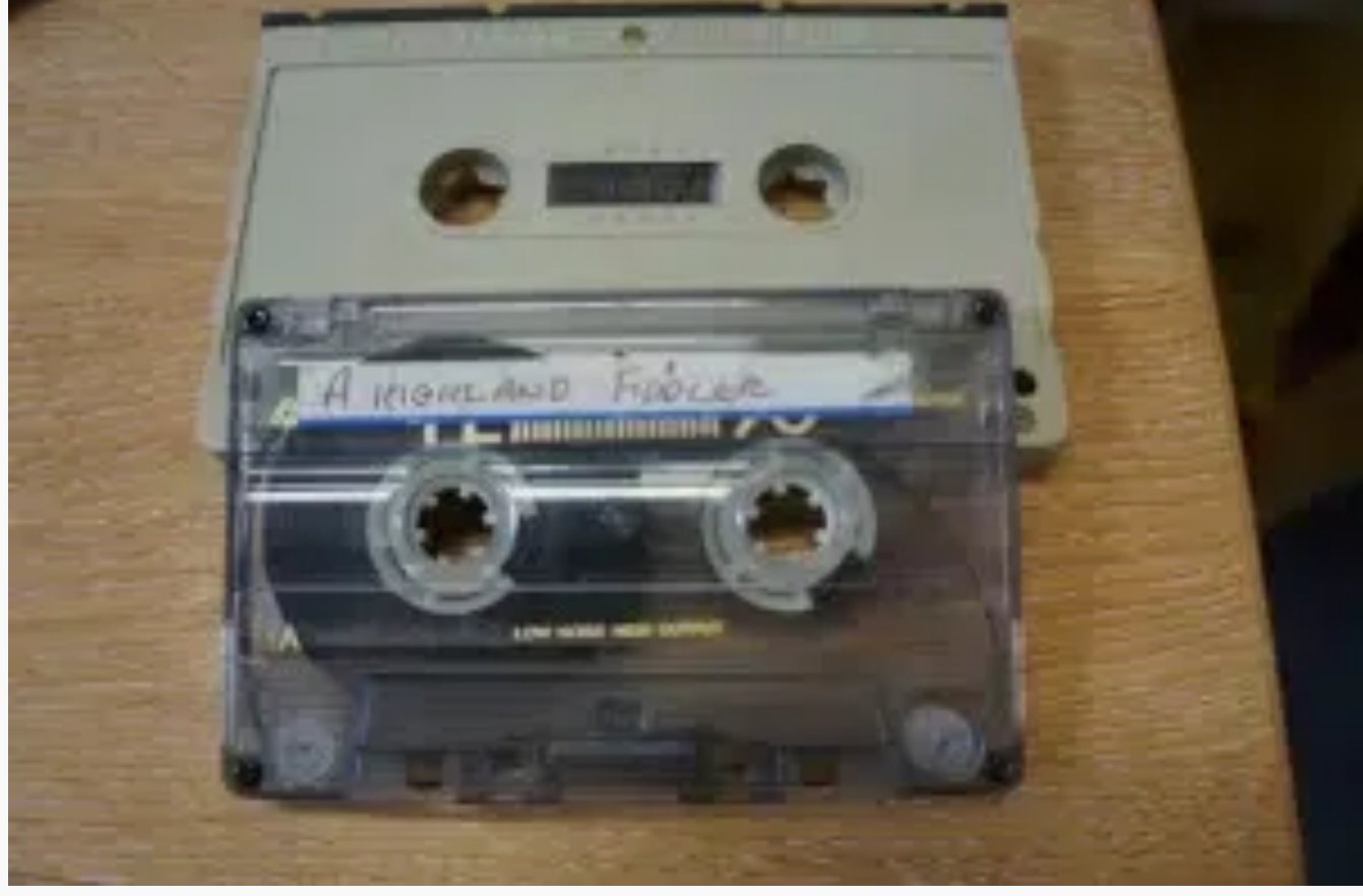
Grundig DC-International compared to standard compact cassette
